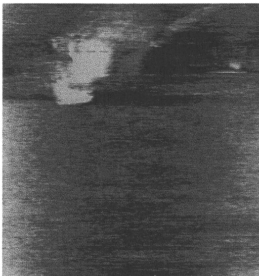
Figure 2. Constant force SFM image of (\text{CH}_3\text{O})_3\text{Si}(\text{CH}_2)_3\text{NH}_2 reflux-treated \text{SiO}_2/\text{Si}(111) . Scan size is 900 x 900 nm and Z-range is 5 nm.
